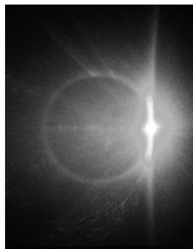
Figure 3. The scattering corona changed to a scattering cone, when the pump beam read out the written refractive index gratings under the angle \theta . The picture shows the projection of the holographic scattering cone on a screen behind the sample, a c-cut of [\text{Ru}(\text{NH}_3)_5\text{NO}]\text{Cl}_3 \cdot \text{H}_2\text{O} (thickness d = 0.24 \text{ mm} ), after illumination with 458 \text{ nm} ( Q = 500 \text{ J cm}^{-2} , \mathbf{E} \parallel \mathbf{a} , \mathbf{k} \parallel \mathbf{c} ) for a read-out angle of \theta = 6^\circ at T = 100 \text{ K} .
